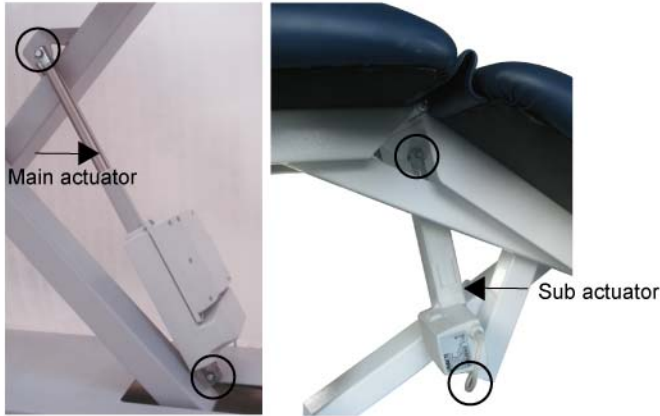
The clamp-spring at both-end of the main actuator
