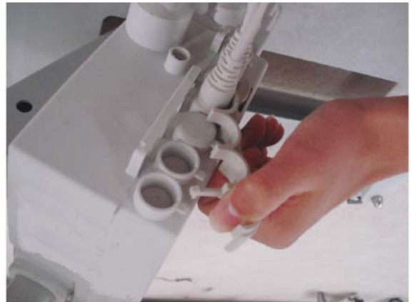
Remove the shielded cable cover
