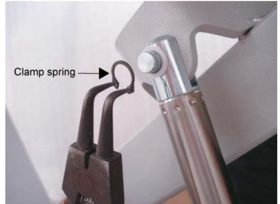
Remove the clamp spring and the bolt
