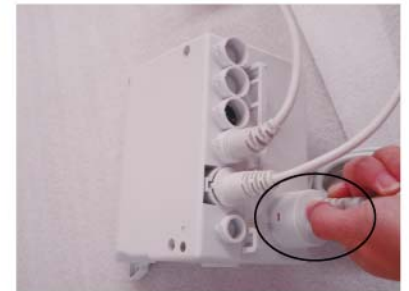
Unplug the power cable from the control-box, then plug in again.
