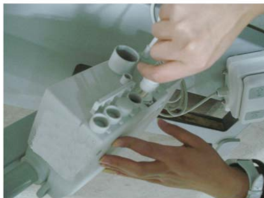
Remove the actuator cables from the control-box
